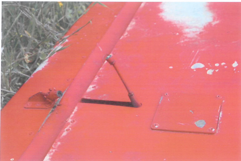
Photo 12: Trim Tab Elevator Connection
