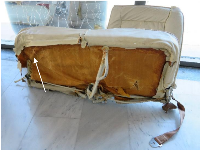
Photo 21: Rear seat frame showing the missing part of the right seat frame (white arrow).
