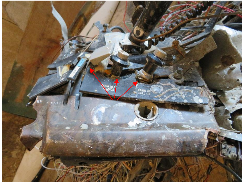
Photo 16: Right Instrument panel, the three switches right bending.
