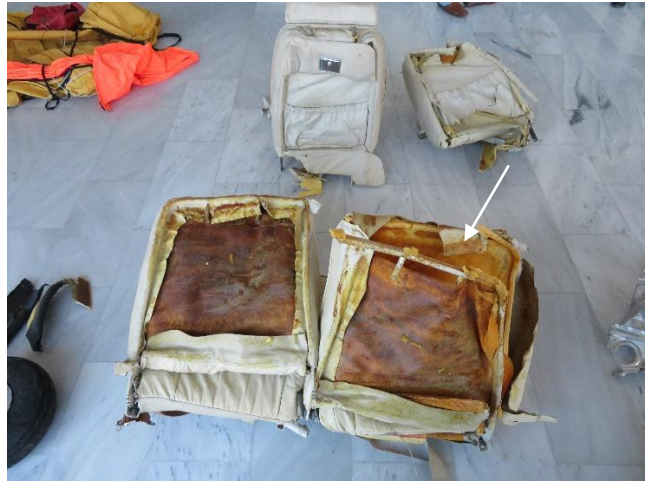
Photo 22: The frame of the rear seat back, where fracture and deformation of the right back frame the left can be seen.
