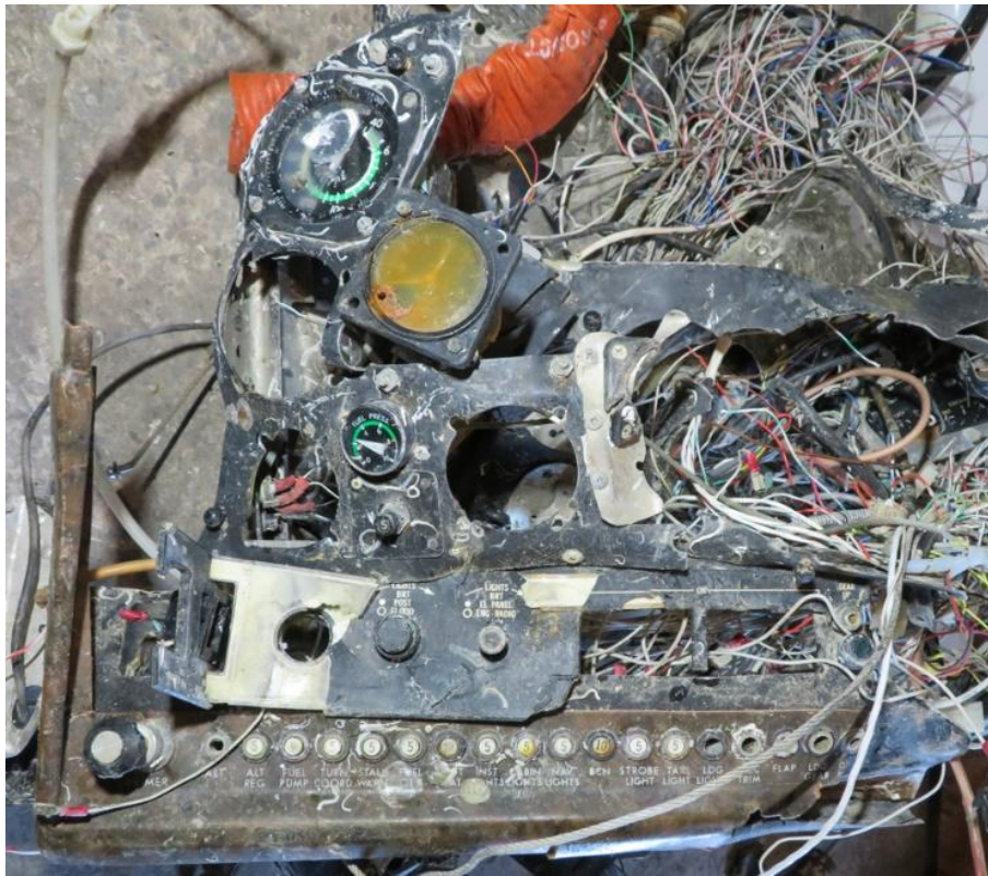
Photo 14: Part of recovered left Instrument panel.
