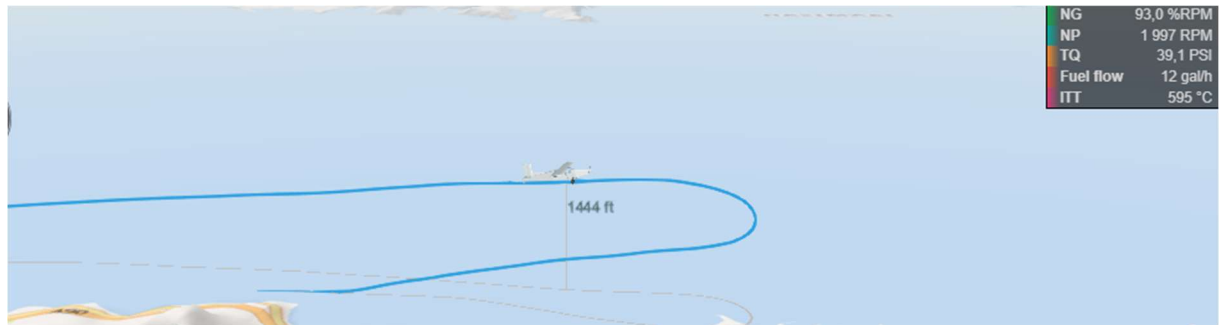
Figure 4: Characteristics of engine performance of the aircraft at a height of 1444 ft.
